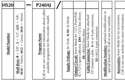
Example: HS20.5-P240AJ/8-30 - 1/2" shaft bore, P240AJ program, 8-30vdc, push/pull output, attached 10' cable
