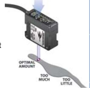
**D. Two-Point AUTOSET Mode** – Use this mode to establish upper and lower limits. When monitoring the target luminescence using the analog output, this mode will set your upper and lower control limits at specific points on the analog output scale. This is the most sensitive mode for detection of low contrast differences in two UV luminescent materials. An example would be glue on a white paper envelope, where both the glue and the paper have optical brighteners present.
