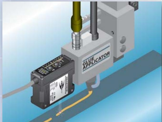
*Glue Measurement for Feedback Loop*
