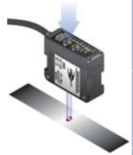
**B. Dark State AUTOSET Mode** – With background in view, the sensor samples the signal level from the background and sets the switching threshold just above that signal level. The sensor is sensitive to more luminescent materials in this mode. This mode is useful in solving many common applications. The analog output can be used to provide feedback of target brightness level for control applications in this mode as well.
