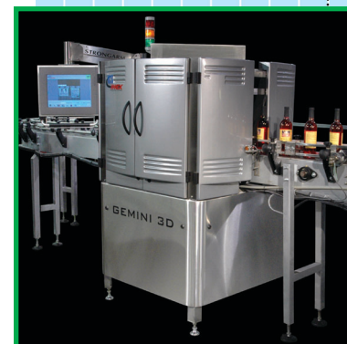
The Gemini 3D (above), an unoriented-label inspector, is the latest ICS Inex machine to use the RetroSmart proximity sensor (below), a simple-to-use device that can detect the presence of clear containers.
